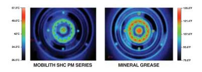
As illustrated in the thermal images above, Mobilith SHC PM Series exhibits exceptional friction control, resulting in lower bearing temperatures in FE-9 bearing tests compared with mineral oil-based products.
