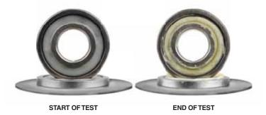
In water washout testing (ASTM D 12264), Mobilith SHC PM Series delivers outstanding protection, with significantly less grease loss compared to competitive products. Effective water washout resistance can translate to extended equipment component life through rust and corrosion protection.
