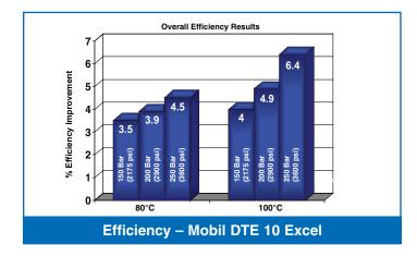
This demonstration shows the impact that fluid formulation and physical characteristics can have on overall hydraulic efficiency. But hydraulic efficiency is not an end goal in and of itself. This additional pumping efficiency can translate into energy savings, as measured by fuel or electricity consumption, or into decreases in time to complete a work cycle in hydraulically powered equipment.
