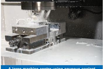
A large machine center using aqueous coolant
